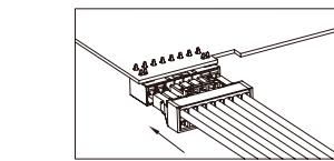
EN The mounting and dismounting of the removable terminal block are shown in the figures on the right side.
